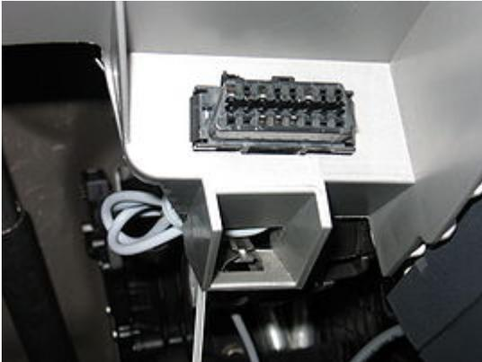
The OBD-II specification provides for a standardized hardware interface—the female 16-pin (2x8) J1962 connector. Unlike the OBD-I connector, which was sometimes found under the hood of the vehicle, the OBD-II connector is nearly always located on the driver's side of the passenger compartment near the center console or driver footwell. SAE J1962 defines the pinout of the connector as:
